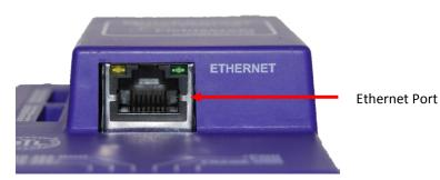
The Ethernet Port is used both for BACnet Ethernet and BACnet/IP communications. It is also used for configuring the Router from a Web page. Follow the steps below to connect the Router to a BACnet network and optionally to a PC for configuration purposes:
