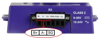
Connect to the 3 pins on the left-hand-side of the 6 pin connector as shown.
