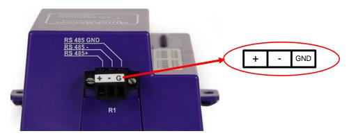
The following Baud Rates are supported on the R1 Port: 110, 300, 600, 1200, 2400, 4800, 9600, 19200, 20833, 28800, 38400, 57600, 76800, 115200
