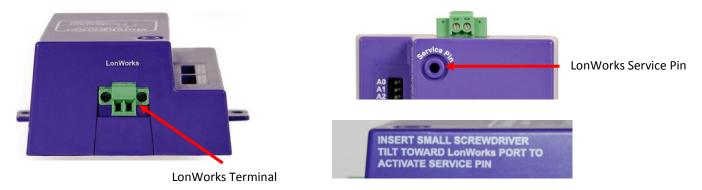
To commission the QuickServer LonWorks port, insert a small screwdriver in the commissioning hole on the face of the QuickServer's enclosure to access the Service Pin. See the instructions on the QuickServer as to which way to toggle the screwdriver during commissioning.
