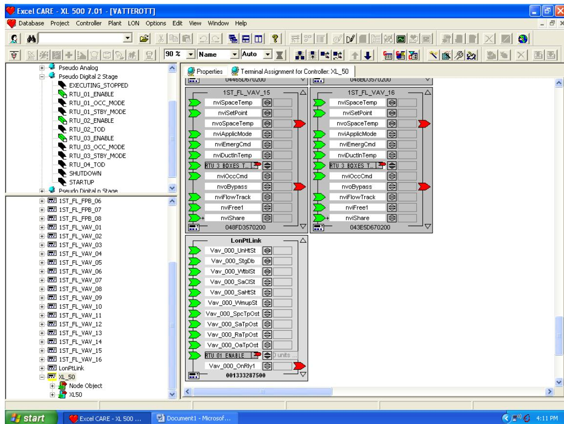
Next, open up the nv points bound from your controller under the controller in the network tree and set your nvo points to Ackd bindings in the service type as shown below. Care automatically defaults to unacknowledged bindings.
