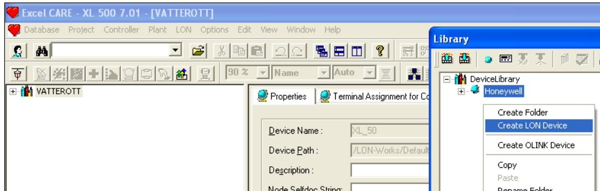
Connect to the Lon side of the PT Link using the Lon network interface cable and set Care to Onnet.
